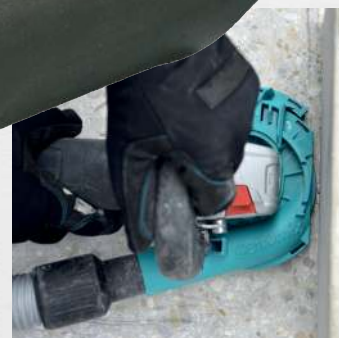
Practical segment opening for precise working on edges
