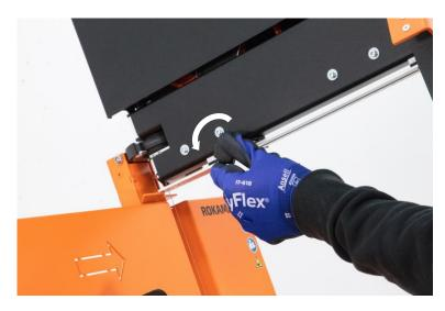
Loosen the star knob screw of the upper height stop.
