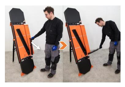
Fold down the right-hand support bracket completely.
