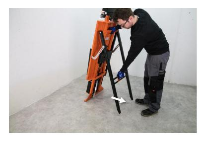
Extend the folding foot as far as it will go to set up the cutter.
