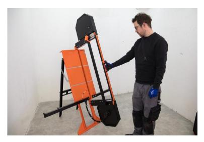
The insulation cutter is now ready for use (provided a charged CAS battery is inserted and the motor has been switched on).
