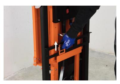
Pull the lock on the folding foot upwards.
