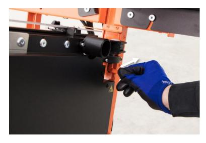
Tighten the lower clamping lever of the cutting bow.
