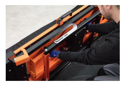
Hold the tool at the back of the main carrier.
