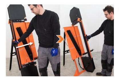
Position the cutting bow at  $0^{\circ}$ .
