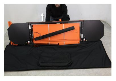
Lift the tool vertically upwards.
