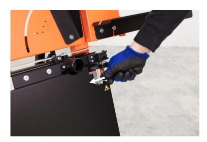
Release the lower clamping lever of the cutting bow.
