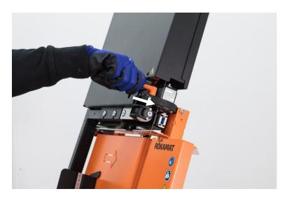
Release the upper clamping lever of the cutting bow.
