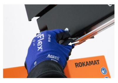
Pull out the upper fixing bolt.
