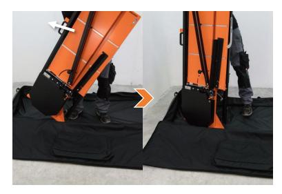
Now stand the tool upright using the support leg of the main carrier.
