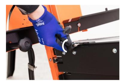
Tighten the star knob screw of the lower height stop.
