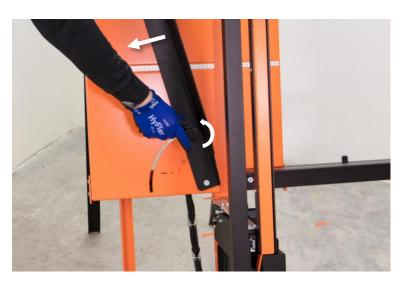
Loosen the star knob screw of the left-hand support bracket and then fold it down.
