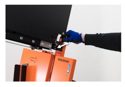
Tighten the upper clamping lever of the cutting bow.
