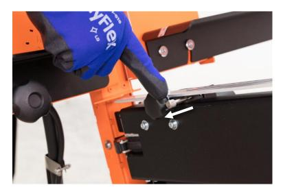
Pull out the lower fixing bolt.
